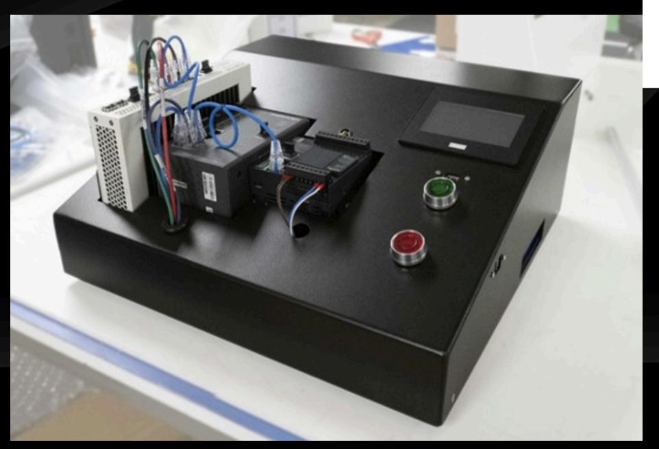
These rugged ICS training kits are constructed with basic inputs and outputs. They are used to familiarize students with Programmable Logic Controller (PLC) and Human Machine Interface (HMI) programming, networking, and communication with the PLC. They also teach ICS protocols, active scanning and network & endpoint manipulation, and attacking & securing ICS networks.
