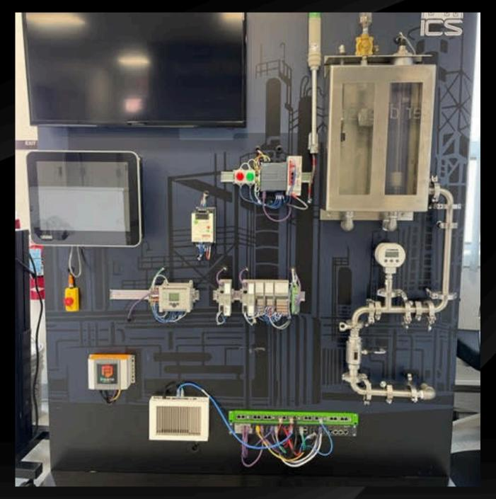
CyberHive is a large custom 5'x6' "wall on wheels display" of an Industrial Control System (ICS) network commonly found in operational technology (OT) environments to support hands-on, unique visual learning objectives. All assets on the wall are configured to simulate a real-world environment, i.e., a water tank that fills and drains according to the student training activity.
